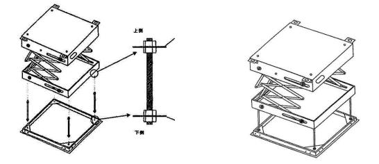
3. Check and ensure the projector motorized lift run well (if there is remote control, please check it) before installation.
